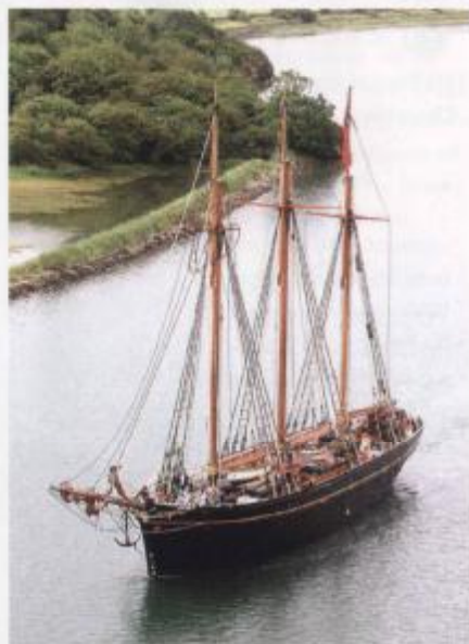
98ft 4in (30m) b Ferguson and Baird, Chester, 1900 Three-masted topsail trading schooner, bought in 1970 by the Maritime Trust, which sold her in 1998 to Bideford man Steve Clark, who restored her. Still sailing, she is part of the NHS Core Collection. CB178
