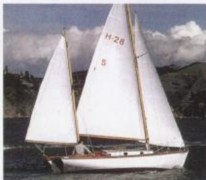
26 H-28 28ft (8.5m) d LF Herreshoff, 1942 "More circumnavigations have been made with the H-28 than any other design." Easy to build, pretty, stable, and with her low-aspect ketch rig, simple, comfortable and seaworthy. CB53
