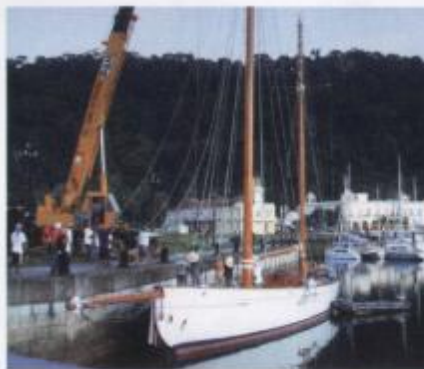
26 H-28 28ft (8.5m) d LF Herreshoff, 1942 "More circumnavigations have been made with the H-28 than any other design." Easy to build, pretty, stable, and with her low-aspect ketch rig, simple, comfortable and seaworthy. CB53
